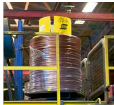
Figure 3. EcoCoil on a turning table.
