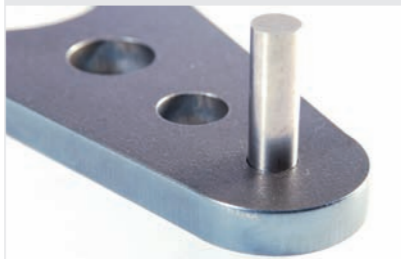
A 20mm pin in a 20mm hole in 12mm steel
